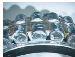
Photo. 6.2 Filling grease into cylindrical roller bearing
