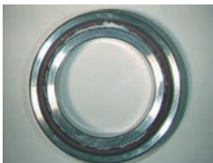
Photo. 6.1 Filling grease into angular contact ball bearing
